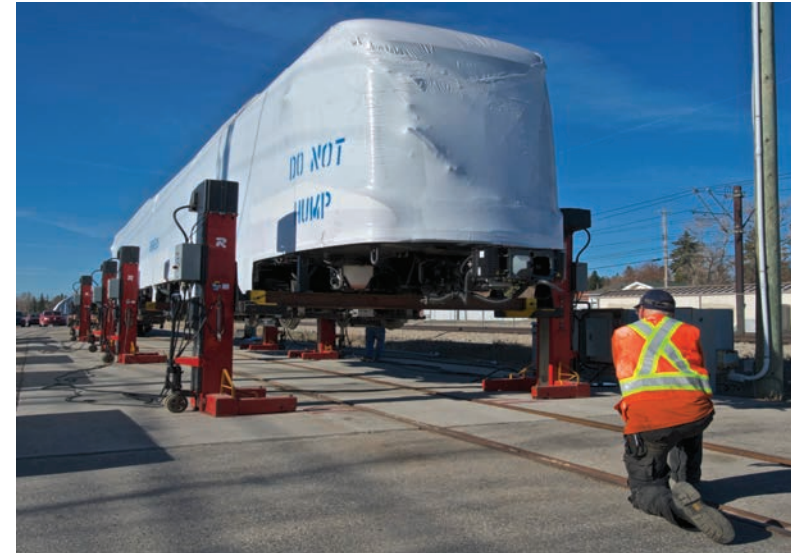
Lowering the car to the rails begins.
