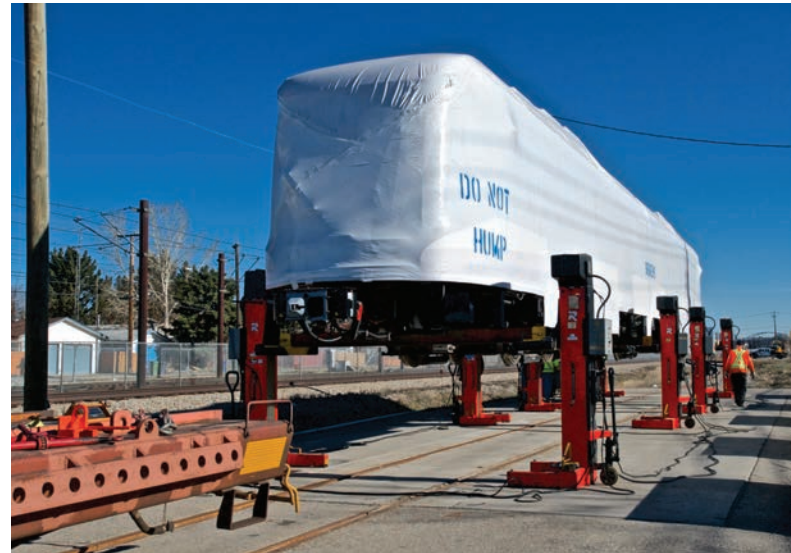
LRV 2442 on jacks as flatcar is pulled away.
