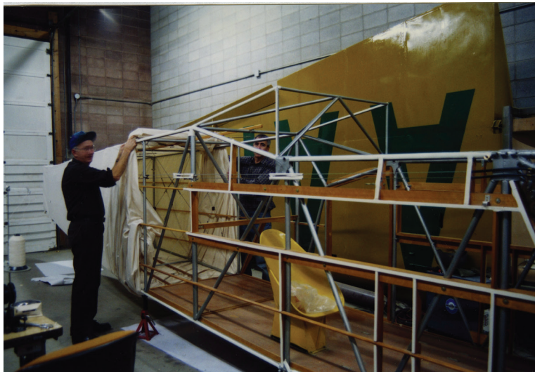
Don Mclean and Clark Seaborn pulling the cotton covering bag over the fuselage. Just as sitting down to pull your socks on, the fuselage had to be raised on a trestle below the cabin, and the tail roller had to be removed to get the bag pulled on.
