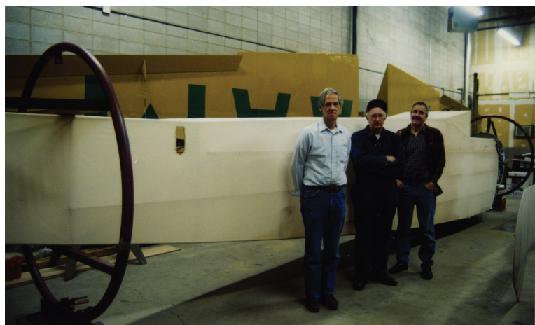
Completed fuselage-covering envelope. Crew left to right, Murray Deines, Don Mclean, Clark Seaborn.
