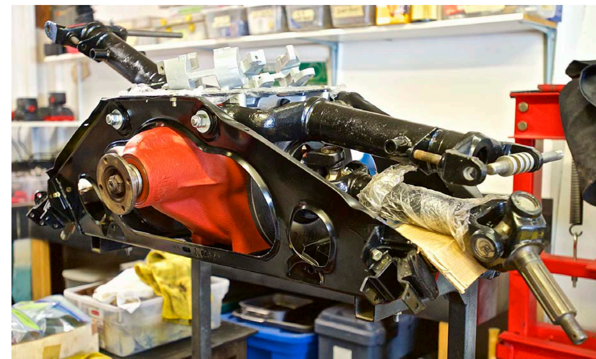
Remanufactured XK-E differential, inboard brakes, suspension arms and axles
