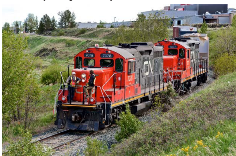
The CN crew control the locomotives with belt packs that are wirelessly linked to the locomotive controls.
