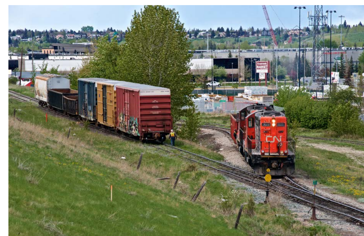
To return safely to the yard, the crew moves the locomotives to the leading end of the train of cars.
